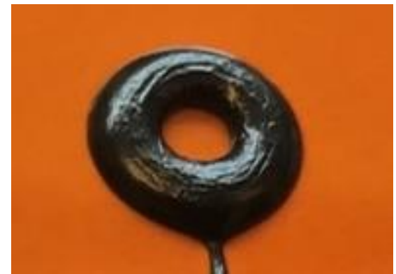
Iron/epoxy 3D printed toroid
